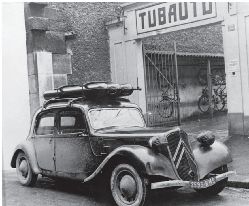
Figure 1. Gazogène -fueled Automobile.
